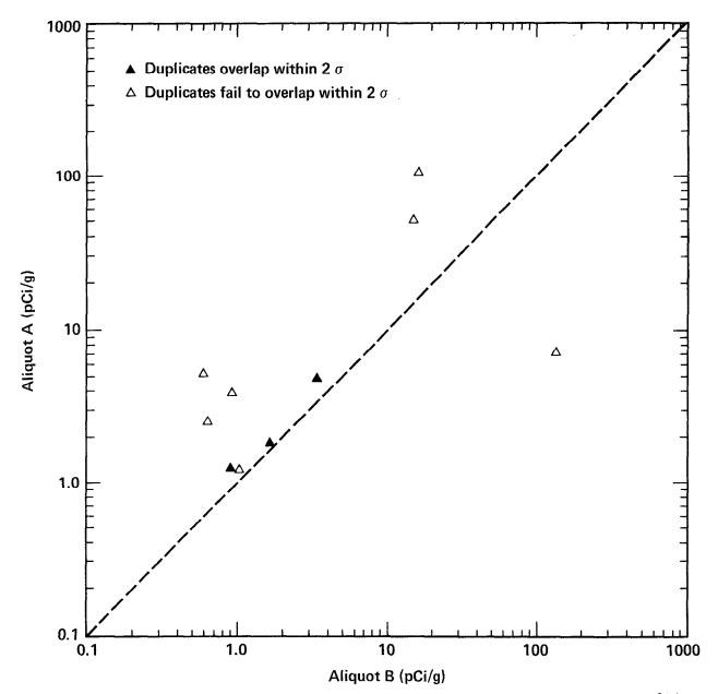
Figure A43. Unacceptable quality control results for duplicate pairs analyzed for <sup>241</sup>Pu in soil by Eberline Instrument Corporation. Broken line represents perfect agreement and is not a fit to the data. Twelve unacceptable pairs involving detections limits are not shown.
