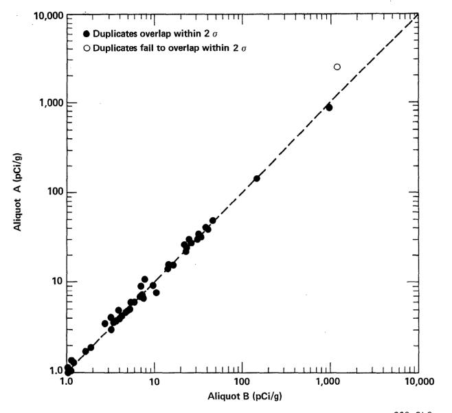
Figure A4. Acceptable quality control results for duplicate pairs analyzed for  $^{239+240}$ Pu in soil by Environmental Analysis Laboratory. Results depicted are for concentrations between 1 and 10,000 pCi/g. Broken line represents perfect agreement and is not a fit to the data. One unacceptable pair is not shown.
