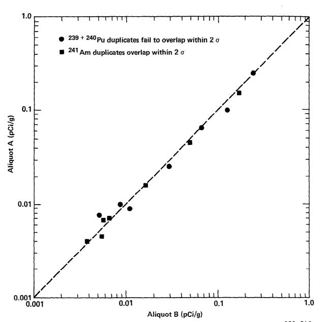
Figure A22. Acceptable quality control results for duplicate pairs analyzed for  $^{239+240}$ Pu and  $^{241}$ Am in marine sediment by Environmental Analysis Laboratory. Broken line represents perfect agreement and is not a fit to the data.
