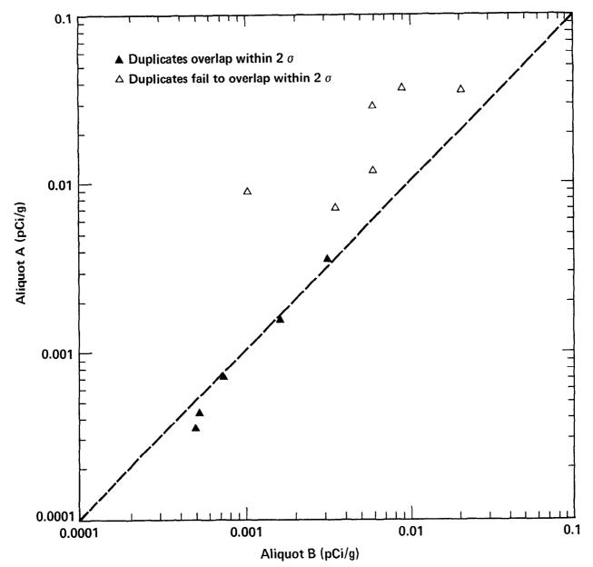
Figure A38. Unacceptable quality control results for duplicate pairs analyzed for 239+240Pu in soil by Environmental Analysis Laboratory. Broken line represents perfect agreement and is not a fit to the data. One acceptable pair involving zero concentrations is not shown.
