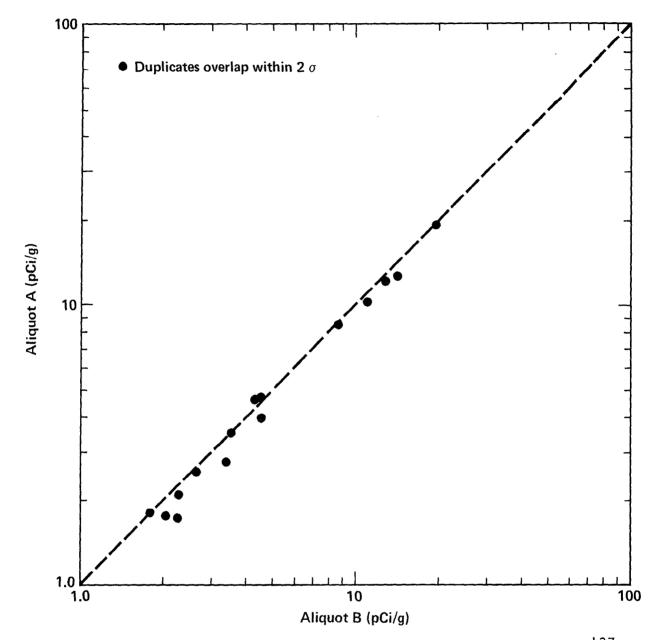
Figure A31. Acceptable quality control results for duplicate pairs analyzed for  $^{137}$ Cs in vegetation by Eberline Instrument Corporation. Broken line represents perfect agreement and is not a fit to the data.
