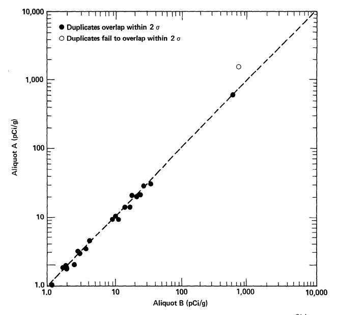
Figure A10. Acceptable quality control results for duplicate pairs analyzed for <sup>241</sup>Am in soil by Environmental Analysis Laboratory. Results depicted are for concentrations between 1 and 10,000 pCi/g. Broken line represents perfect agreement and is not a fit to the data.
