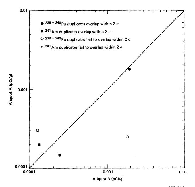
Figure A32. Acceptable quality control results for duplicate pairs analyzed for  $^{239+240p_{u}}$  and  $^{241}Am$  in vegetation by Eberline Instrument Corporation. Broken line represents perfect agreement and is not a fit to the data. Eight acceptable pairs (seven  $^{239+240p_{u}}$ ) and six unacceptable pairs (three  $^{239+240p_{u}}$ ) involving zero or negative concentrations or detection limits are not shown.
