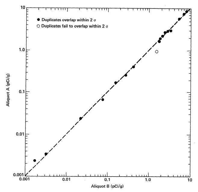
Figure A37. Acceptable quality control results for duplicate pairs analyzed for <sup>241</sup>Am in soil by Laboratory of Radiation Ecology. Broken line represents perfect agreement and is not a fit to the data.
