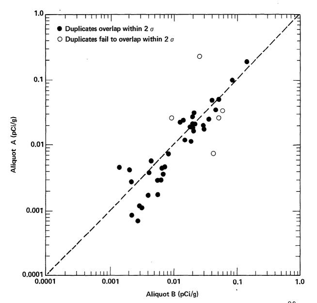
Figure A12. Acceptable quality control results for duplicate pairs analyzed for <sup>90</sup>Sr in vegetation by Environmental Analysis Laboratory. Broken line represents perfect agreement and is not a fit to the data. Three acceptable pairs involving zero concentrations are not shown.
