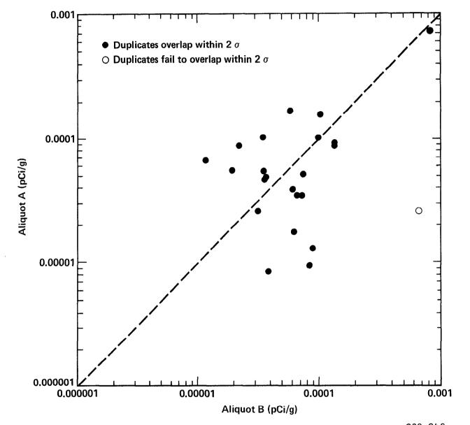
Figure A14. Acceptable quality control results for duplicate pairs analyzed for  $^{239+240}$ Pu in vegetation by Environmental Analysis Laboratory. Broken line represents perfect agreement and is not a fit to the data. Nineteen pairs (eighteen acceptable) involving zero or negative concentrations are not shown.
