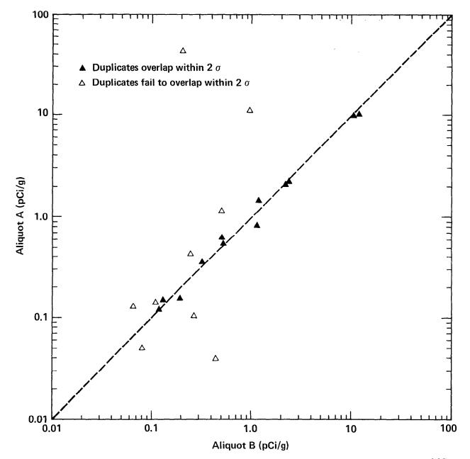
Figure A41. Unacceptable quality control results for duplicate pairs analyzed for 137Cs in soil by Eberline Instrument Corporation. Broken line represents perfect agreement and is not a fit to the data. Three unacceptable pairs involving detection limits are not shown.
