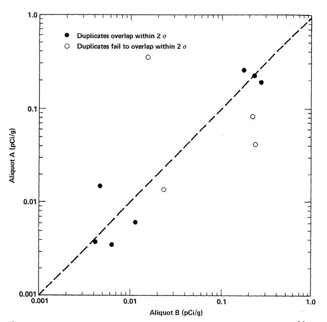
Figure A30. Acceptable quality control results for duplicate pairs analyzed for 90Sr in vegetation by Eberline Instrument Corporation. Broken line represents perfect agreement and is not a fit to the data. Five unacceptable pairs involving detection limits are not shown.
