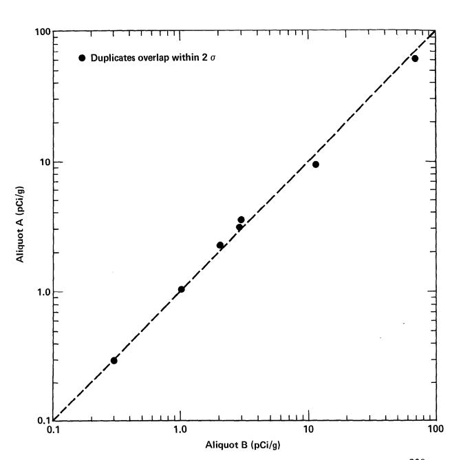
Figure A28. Acceptable quality control results for duplicate pairs analyzed for <sup>238</sup>Pu in soil by Eberline Instrument Corporation. Broken line represents perfect agreement and is not a fit to the data.
