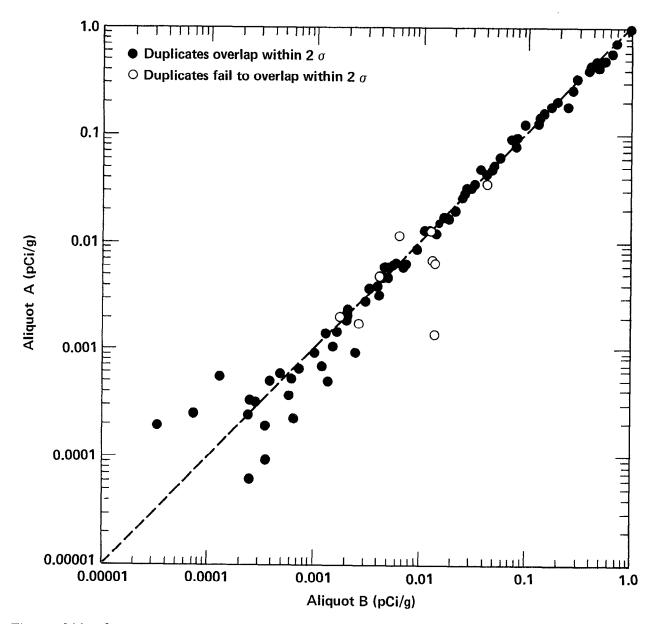
Figure A11. Acceptable quality control results for duplicate pairs analyzed for  $^{241}$ Am in soil by Environmental Analysis Laboratory. Results depicted are for concentrations between 1 x  $10^{-5}$  and 1 pCi/g. Broken line represents perfect agreement and is not a fit to the data. Five pairs (four acceptable) involving zero or negative concentrations are not shown.
