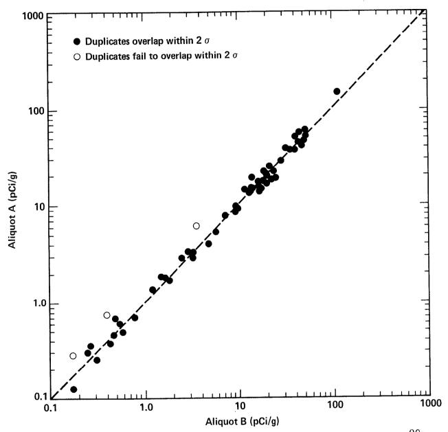
Figure A33. Acceptable quality control results for duplicate pairs analyzed for <sup>90</sup>Sr in soil by Laboratory of Radiation Ecology. Broken line represents perfect agreement and is not a fit to the data. Two unacceptable pairs involving detection limits are not shown.
