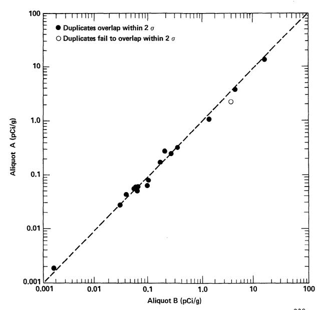
Figure A6. Acceptable quality control results for duplicate pairs analyzed for <sup>238</sup>Pu in soil by Environmental Analysis Laboratory. Broken line represents perfect agreement and is not a fit to the data.
