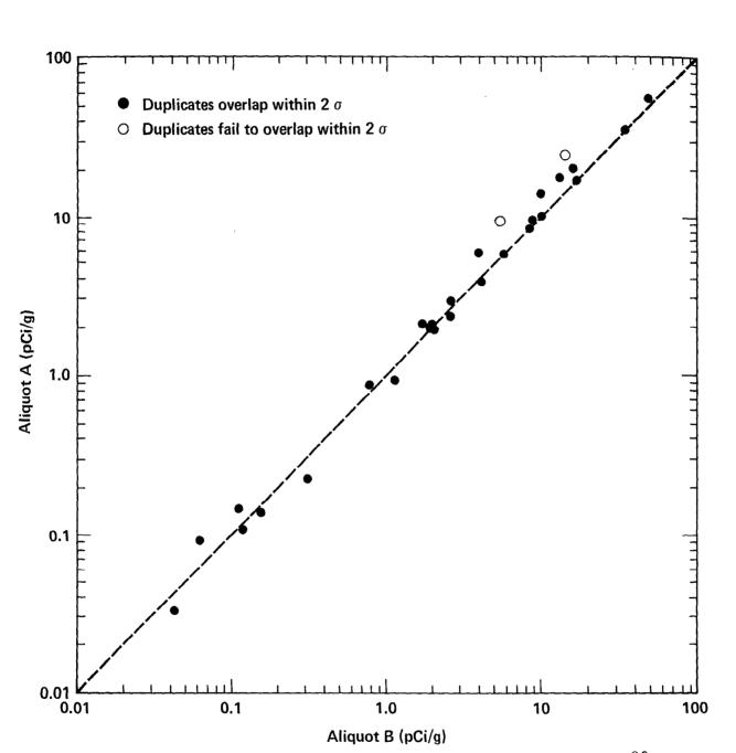
Figure A24. Aceptable quality control results for duplicate pairs analyzed for  $^{90}$ Sr in soil by Eberline Instrument Corporation. Broken line represents perfect agreement and is not a fit to the data.
