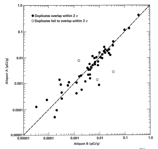
Figure A21. Acceptable quality control results for duplicate pairs analyzed for <sup>241</sup>Am in marine organisms by Environmental Analysis Laboratory. Broken line represents perfect agreement and is not a fit to the data. Seventeen pairs (fifteen acceptable) involving zero or negative concentrations are not shown.
