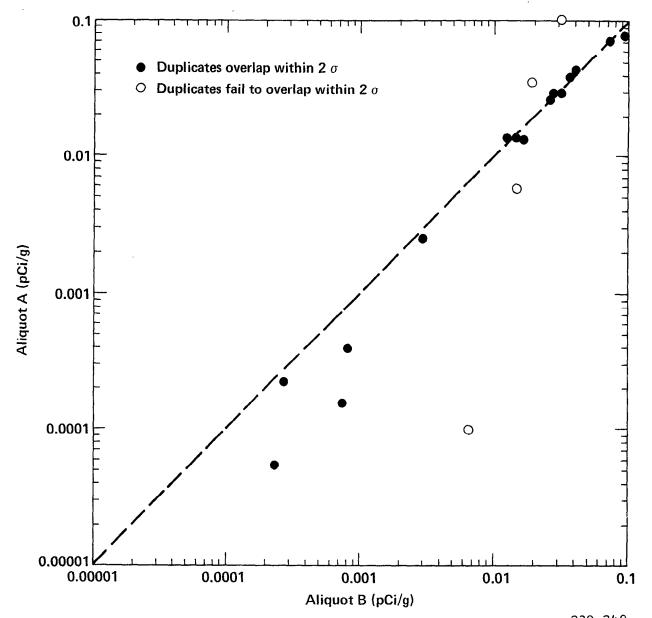
Figure A27. Acceptable quality control results for duplicate pairs analyzed for  $^{239+240}$ Pu in soil by Eberline Instrument Corporation. Results depicted are for concentrations between 1 x 10<sup>-5</sup> and 0.1 pCi/g. Broken line represents perfect agreement and is not a fit to the data.
