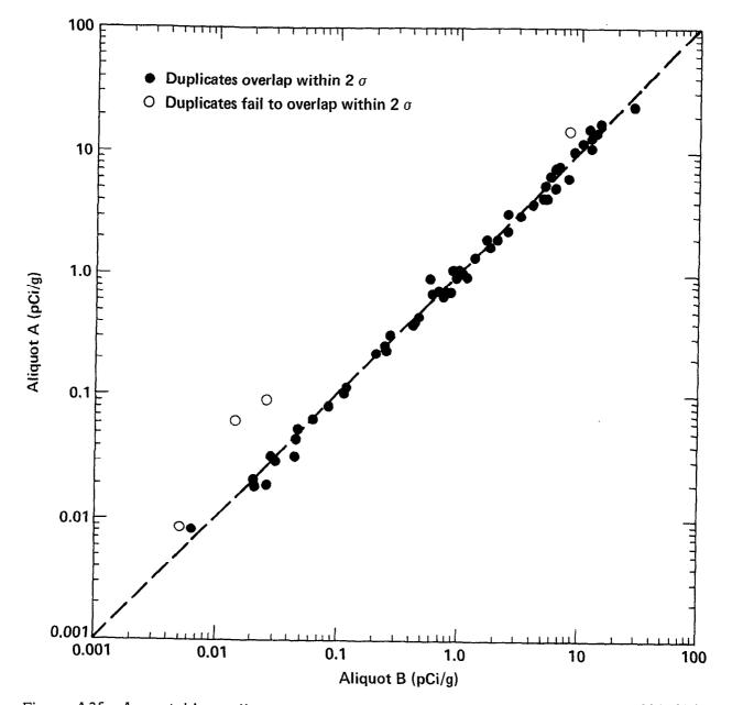
Figure A35. Acceptable quality control results for duplicate pairs analyzed for  $^{239+240}$ Pu in soil by Laboratory of Radiation Ecology. Broken line represents perfect agreement and is not a fit to the data.
