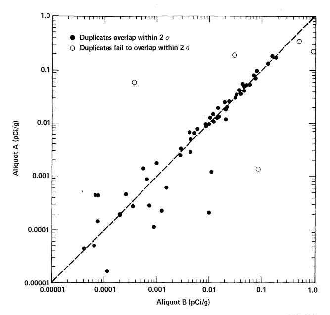
Figure A19. Acceptable quality control results for duplicate pairs analyzed for  $^{239+240}$ Pu in marine organisms by Environmental Analysis Laboratory. Broken line represents perfect agreement and is not a fit to the data. Ten acceptable pairs involving zero or negative concentrations are not shown.
