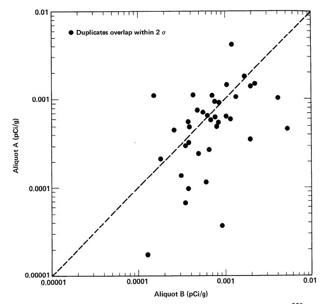
Figure A20. Acceptable quality control results for duplicate pairs analyzed for <sup>238</sup>Pu in marine organisms by Environmental Analysis Laboratory. Broken line represents perfect agreement and is not a fit to the data. Thirty-two acceptable pairs involving zero or negative concentrations are not shown.
