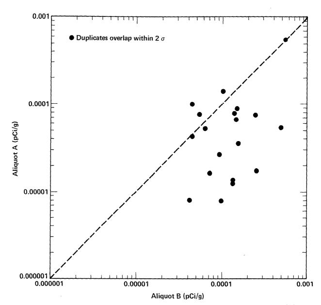
Figure A15. Acceptable quality control results for duplicate pairs analyzed for <sup>241</sup>Am in vegetation by Environmental Analysis Laboratory. Broken line represents perfect agreement and is not a fit to the data. Twenty-five acceptable pairs involving zero or negative concentrations are not shown.
