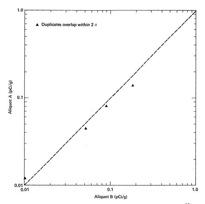
Figure A39. Unacceptable quality control results for duplicate pairs analyzed for  $^{90}$ Sr in marine sediment by Environmental Analysis Laboratory. Broken line represents perfect agreement and is not a fit to the data. Three acceptable pairs involving zero concentrations are not shown.
