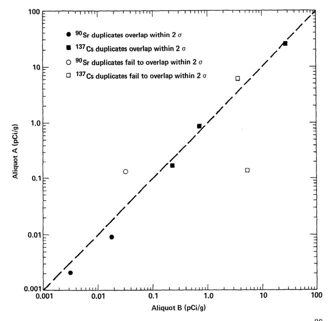
Figure A16. Acceptable quality control results for duplicate pairs analyzed for  $^{90}$ Sr and  $^{137}$ Cs in terrestrial animals by Environmental Analysis Laboratory. Broken line represents perfect agreement and is not a fit to the data. Three acceptable  $^{90}$ Sr pairs involving zero or negative concentrations are not shown.
