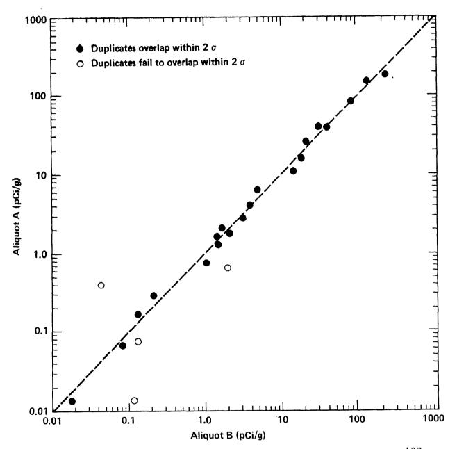
Figure A34. Acceptable quality control results for duplicate pairs analyzed for 137Cs in soil by Laboratory of Radiation Ecology. Broken line represents perfect agreement and is not a fit to the data. Three pairs (two acceptable) involving detection limits are not shown.
