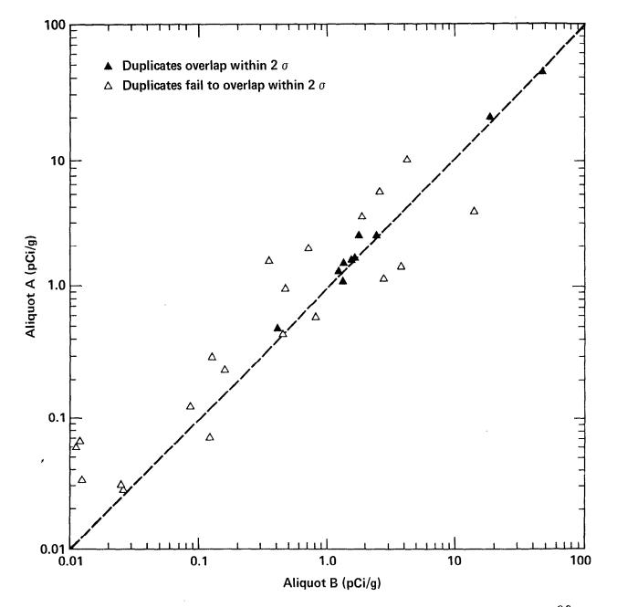
Figure A40. Unacceptable quality control results for duplicate pairs analyzed for  $^{90}$ Sr in soil by Eberline Instrument Corporation. Broken line represents perfect agreement and is not a fit to the data. Two unacceptable pairs involving negative concentrations are not shown.
