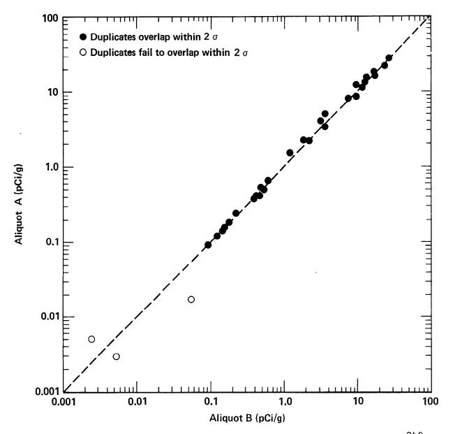
Figure A8. Acceptable quality control results for duplicate pairs analyzed for  $^{240}$ Pu in soil by Environmental Analysis Laboratory. Broken line represents perfect agreement and is not a fit to the data.
