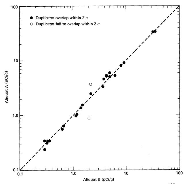
Figure A13. Acceptable quality control results for duplicate pairs analyzed for  $^{137}Cs$  in vegetation by Environmental Analysis Laboratory. Broken line represents perfect agreement and is not a fit to the data.
