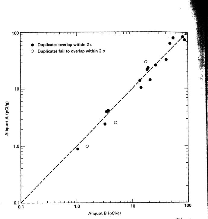
Figure A36. Acceptable quality control results for duplicate pairs analyzed for <sup>241</sup>Pu in soil by Laboratory of Radiation Ecology. Broken line represents perfect agreement and is not a fit to the data.
