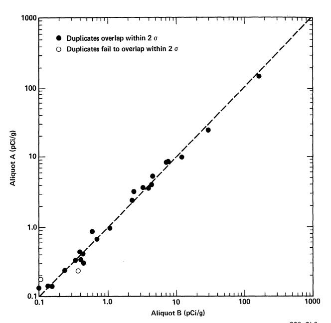
Figure A26. Acceptable quality control results for duplicate pairs analyzed for  $^{239+240}$ Pu in soil by Eberline Instrument Corporation. Results depicted are for concentrations between 0.1 and 1000 pCi/g. Broken line represents perfect agreement and is not a fit to the data.
