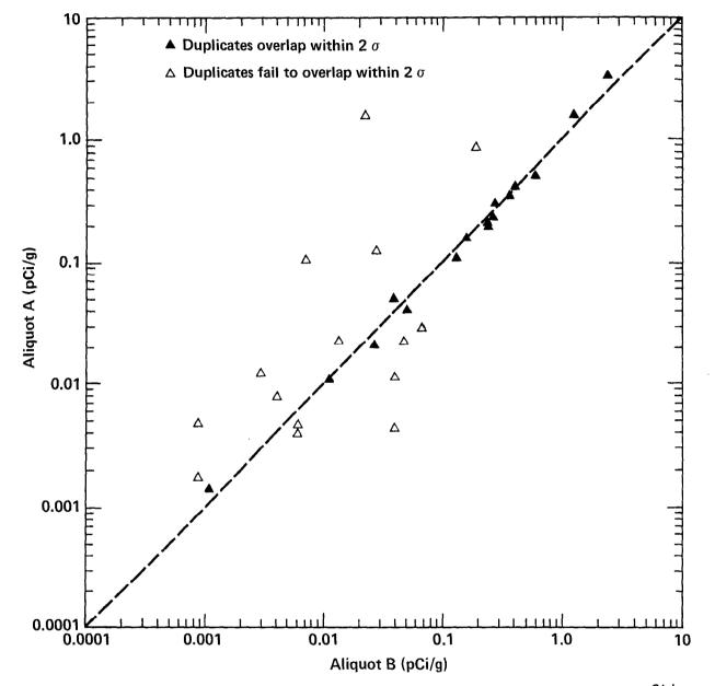
Figure A44. Unacceptable quality control results for duplicate pairs analyzed for <sup>241</sup>Am in soil by Eberline Instrument Corporation. Broken line represents perfect agreement and is not a fit to the data. Five unacceptable pairs involving negative concentrations or detection limits are not shown.
