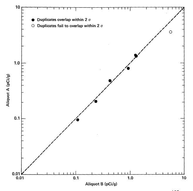
Figure A25. Acceptable quality control results for duplicate pairs analyzed for  $^{137}$ Cs in soil by Eberline Instrument Corporation. Broken line represents perfect agreement and is not a fit to the data.
