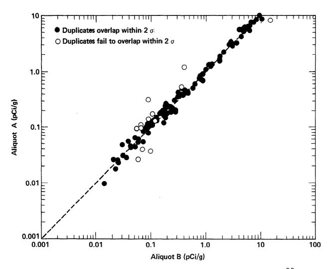
Figure A2. Acceptable quality control results for duplicate pairs analyzed for 90Sr in soil by Environmental Analysis Laboratory. Results depicted are for concentrations between 1 x  $10^{-3}$  and 10 pCi/g. Broken line represents perfect agreement and is not a fit to the data.
