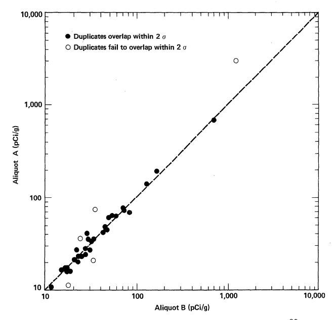
Figure A1. Acceptable quality control results for duplicate pairs analyzed for  $^{90}$ Sr in soil by Environmental Analysis Laboratory. Results depicted are for concentrations between 10 and 10,000 pCi/g. Broken line represents perfect agreement and is not a fit to the data.
