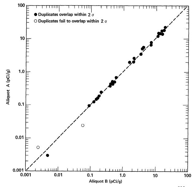
Figure A7. Acceptable quality control results for duplicate pairs analyzed for  $^{239}$ Pu in soil by Environmental Analysis Laboratory. Broken line represents perfect agreement and is not a fit to the data.
