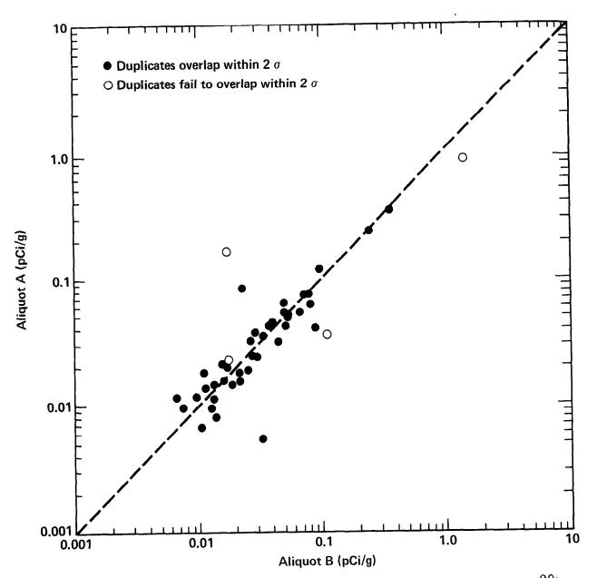
Figure A18. Acceptable quality control results for duplicate pairs analyzed for <sup>90</sup>Sr in marine organisms by Environmental Analysis Laboratory. Broken line represents perfect agreement and is not a fit to the data. Twenty-five acceptable pairs involving zero concentrations are not shown.
