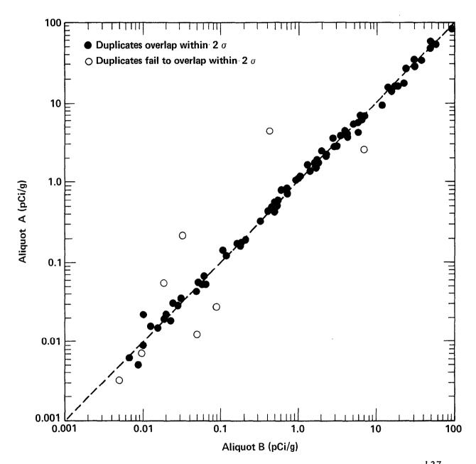
Figure A3. Acceptable quality control results for duplicate pairs analyzed for  $^{137}$ Cs in soil by Environmental Analysis Laboratory. Broken line represents perfect agreement and is not a fit to the data. Two pairs (one acceptable) involving zero concentrations are not shown.
