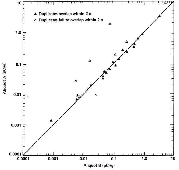
Figure A42. Unacceptable quality control results for duplicate pairs analyzed for  $^{239+240}$ Pu in soil by Eberline Instrument Corporation. Broken line represents perfect agreement and is not a fit to the data.
