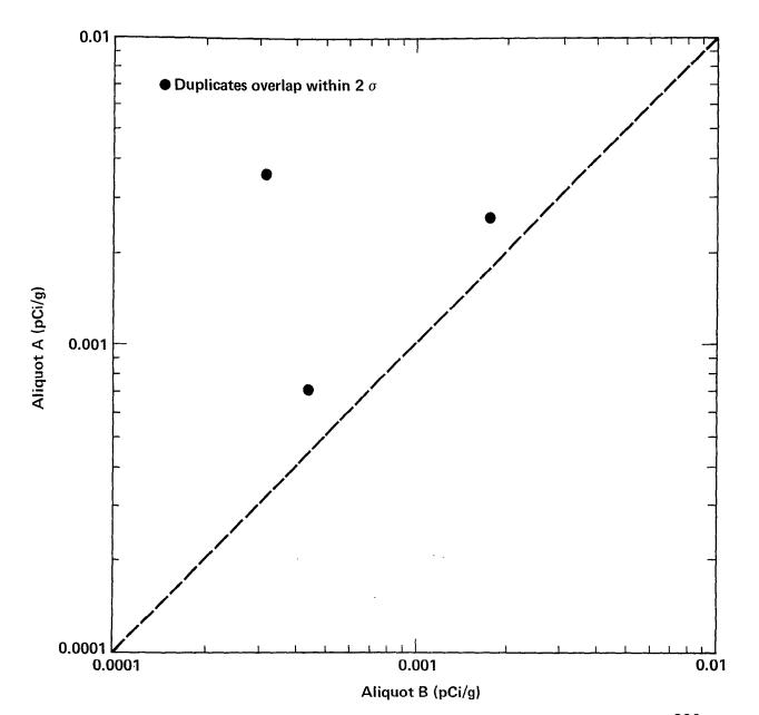
Figure A23. Acceptable quality control results for duplicate pairs analyzed for <sup>238</sup>Pu in marine sediment by Environmental Analysis Laboratory. Broken line represents perfect agreement and is not a fit to the data. Four acceptable pairs involving zero or negative concentrations are not shown.
