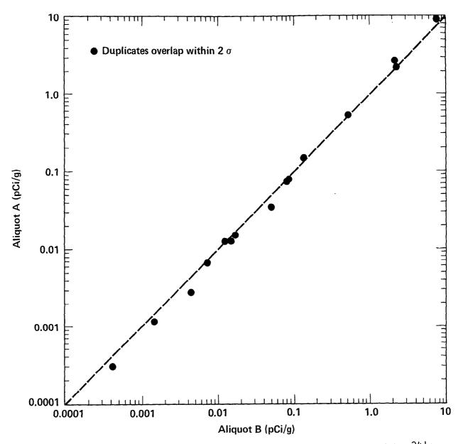
Figure A29. Acceptable quality control results for duplicate pairs analyzed for <sup>241</sup>Am in soil by Eberline Instrument Corporation. Broken line represents perfect agreement and is not a fit to the data.
