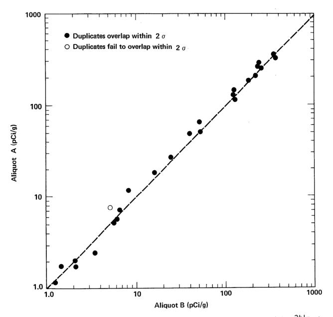
Figure A9. Acceptable quality control results for duplicate pairs analyzed for <sup>241</sup>Pu in soil by Environmental Analysis Laboratory. Broken line represents perfect agreement and is not a fit to the data.
