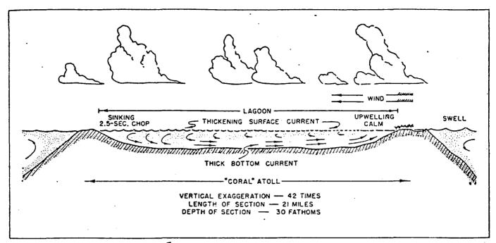
FIGURE 28-Nature of wind-driven overturning circulation (schematic).
