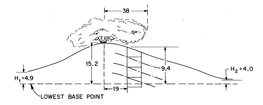
Fig. 1. Schematic representation of a desert mound. Samples were taken at middistance from stem of shrubbery and vertical to the lowest base point plane. Curve line suggests an alternative sampling mode. H<sub>1</sub> = highest point of mound base; H<sub>2</sub> = height of mound base at lowest point from sampled area of mound. Values are in centimeters.
