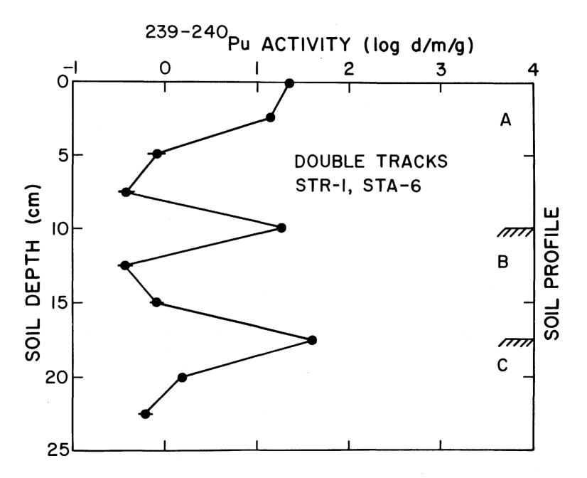
Fig. 2. Distribution of plutonium in Double Tracks soil profile
