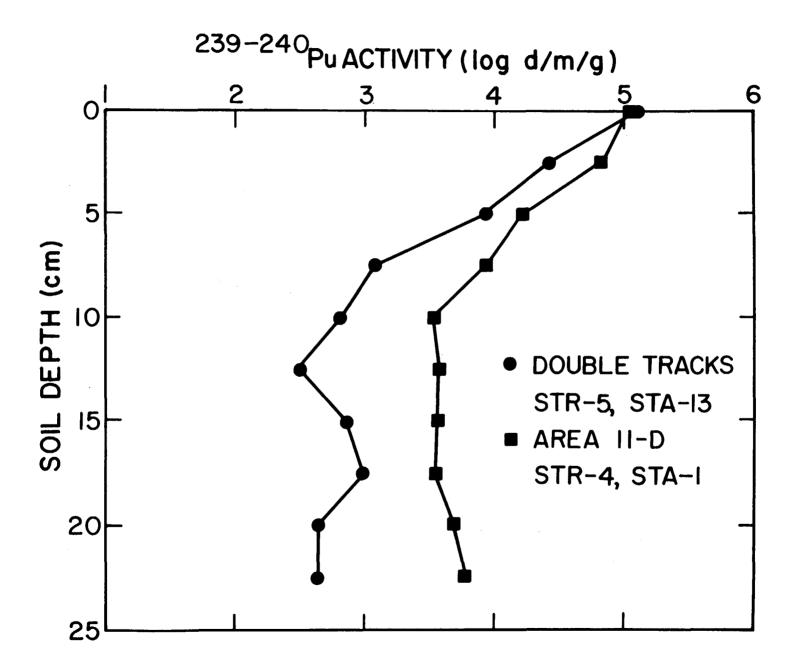
Fig. 3. Distribution of plutonium in top 25 cm of soil.
