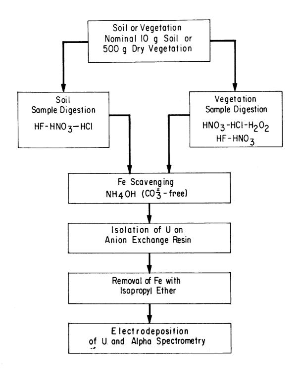
FIGURE 1. FLOW CHART OF TENTATIVE PROCEDURE TO ISOLATE ALPHA SPECTROMETRICALLY PURE U.
