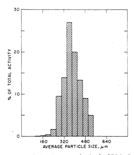
Figure 4. Activity vs granule size for Bikini ash.
