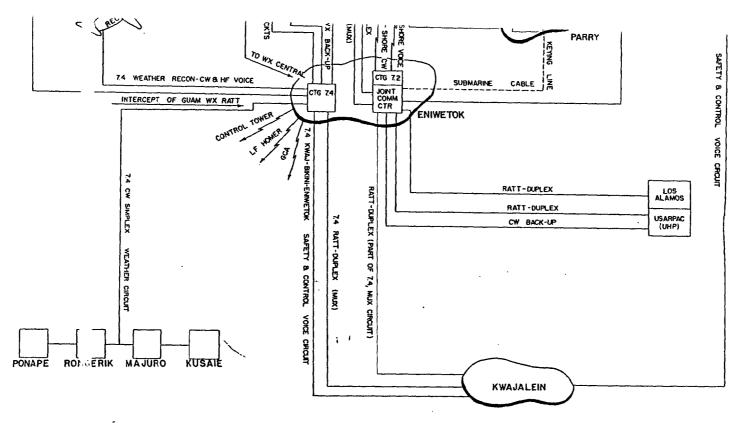
PRINCIPLE TASK FORCE HF RADIO CIRCUITS L-I-I
