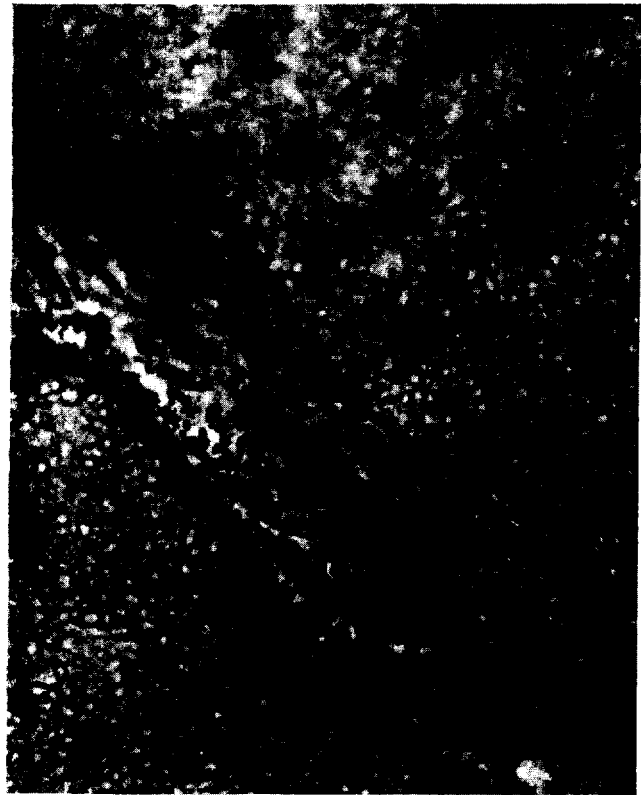
FIG. 2.—A serially etched cellulose nitrate autoradiograph of trabecular bone from mouse, injected with 0.1 \mu Ci ionic ^{239}\text{Pu} , which shows surface alpha tracks. 100 \times .
